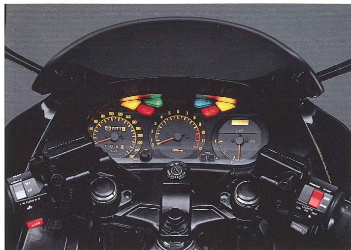
Fairing "cockpit" contains comprehensive instrumentation. Speedometer, rev-counter, large fuel gauge and a digital clock. Carburettor choke control is also conveniently positioned there.
