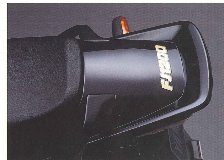
The tail cowl has separate grab-bars on each side, which allows a flat surface on top. Combined with the lip of the rear spoiler, this provides a secure location for soft luggage.
