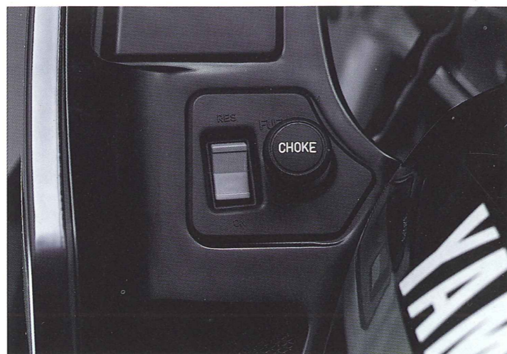
Touring riders will appreciate the provision of an electric fuel reserve switch, located within the fairing cockpit for easy operation. It provides that vital "safety margin" between fuel stops.
