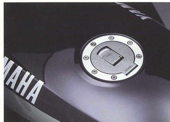
The 22-litre fuel tank has a flush-fitting, aircraft-type filler cap. This permits a flat upper surface to the tank which touring riders will be able to utilise for mounting a tanktop bag.
