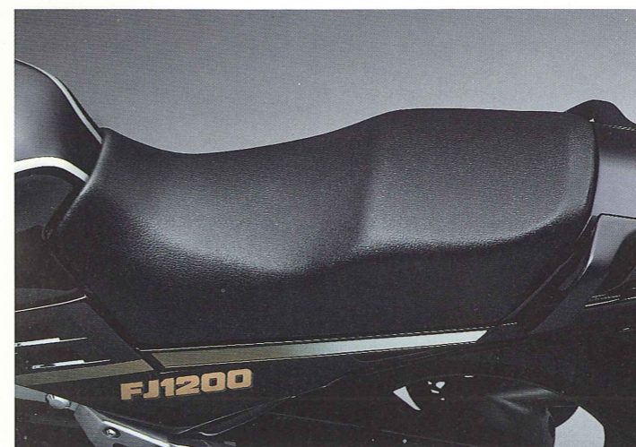
The deeply-padded, seat has been re-designed so that its rear section is flatter. This locates the passenger more firmly under heavy braking.
