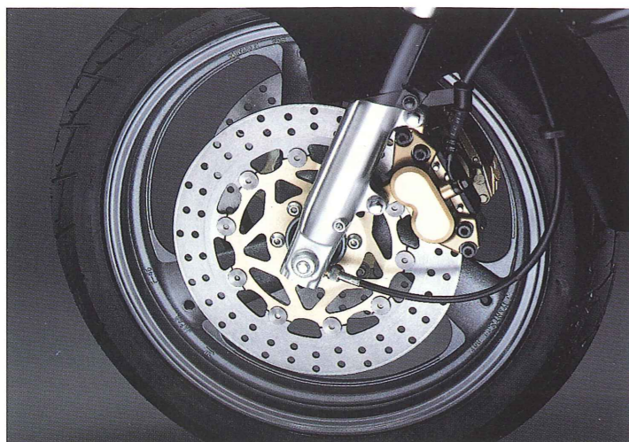
Front wheel and brakes feature dual 298mm floating-type discs with four-pot opposed-piston calipers, mounted to 17-inch, triple hollow-spoke, racing-type wheel.
