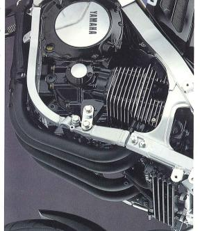
Engine/orthogonal engine mounting
