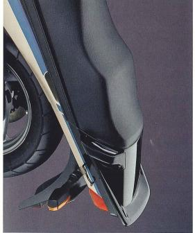
Rider and passenger comfort is of paramount importance on any long-distance machine. Deeply padded and featuring dual contours, the FJ's seat will carry you and your passenger in luxury for hour after hour. And for reduced pillion footrest vibration the silencer is now mounted on a separate
