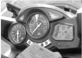
Left: All instrumentation is large and easy to read. The oversized LCD readouts on the right side were especially appreciated, as they can also be read at a glance: Clock, fuel level, engine temp., two tripmeters, odometer, plus diagnostic displays. It's a model of a well-organized dash. Note the big turn signal indicators at the top—you can't miss them.
